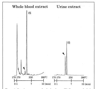
**Figure 4.** Gas chromatograms for the headspace SPME extracts of whole blood and urine samples obtained 150 min after oral administration of 30 mg diphenhydramine–HCl. In each vial, 1.8  $\mu$ g of orphenadrine was spiked as the internal standard. The arrows show the peaks of diphenhydramine. The vertical scale of the whole blood extract is 32 times higher than that of the urine extract.
